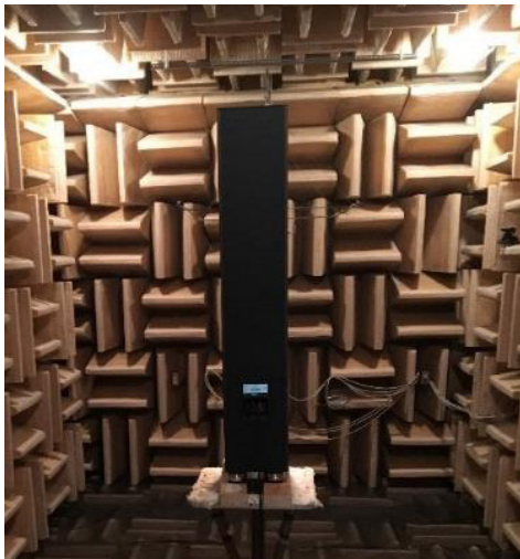
FIGURE 3 – TESTING ISOACOUSTICS IN THE ANECHOIC CHAMBER AT THE NRC
